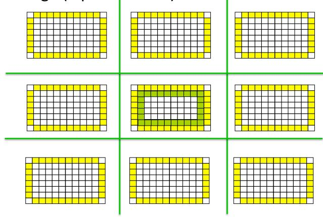
Provide access to remote data through a halo exchange (9 point with trick)
