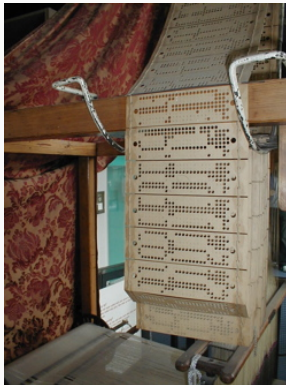
Figure 1: Late 1800s, Jacquard Machine: Threads and Warps
