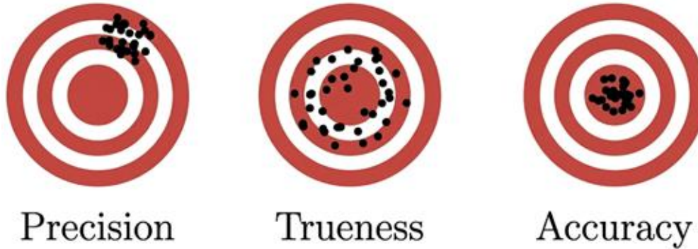
FIGURE 2.3 – Illustration of the concepts of precision, trueness, and accuracy in the context of numerical computation. Each black point represents the result of an execution. These points coincide if the execution is deterministic. Accuracy is a strong property that requires both precision – that the empirical results are not too far from each other – and trueness – that the empirical results is centered on the theoretical result.
