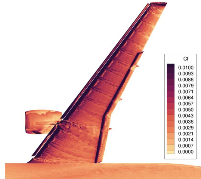
Fig. 12 Wing planform view showing contours of the skin friction magnitude.
