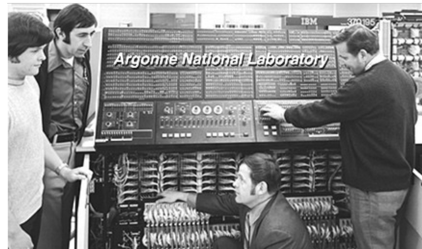
IBM 370/195 18.5 MHz (54 ns clock cycle)
