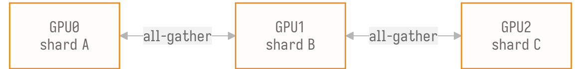
Fig: FSDP / ZeRO — params sharded, all-gathered just-in-time per layer
