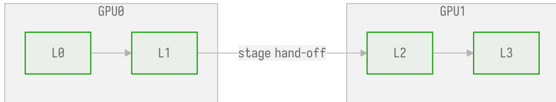
Fig: Pipeline Parallel — layer stack split into stages; micro-batches pipelined
