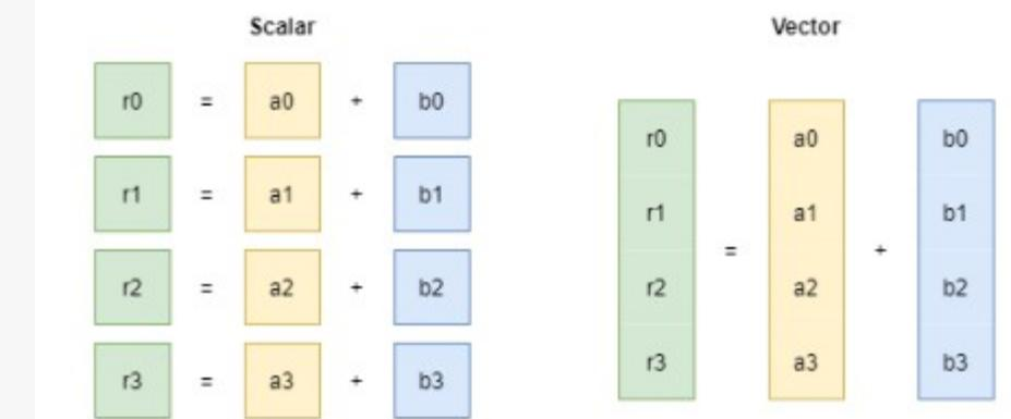
Data parallel devices such as GPUs, SIMD CPUs and other accelerators are vector processors.
