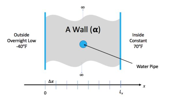
You keep the inside temperature of the house always at 70 degrees F. But, there is an overnight storm coming. The outside temperature is expected to drop to -40 degrees F for 15.5 hours. Will your pipes freeze before the storm is over?
