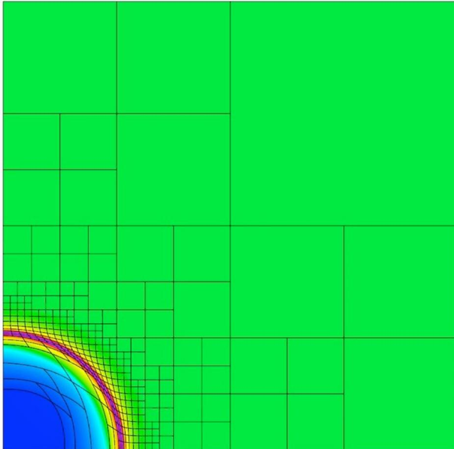
*Adaptive, viscosity-based refinement and derefinement. 2<sup>nd</sup> order Lagrangian Sedov*
