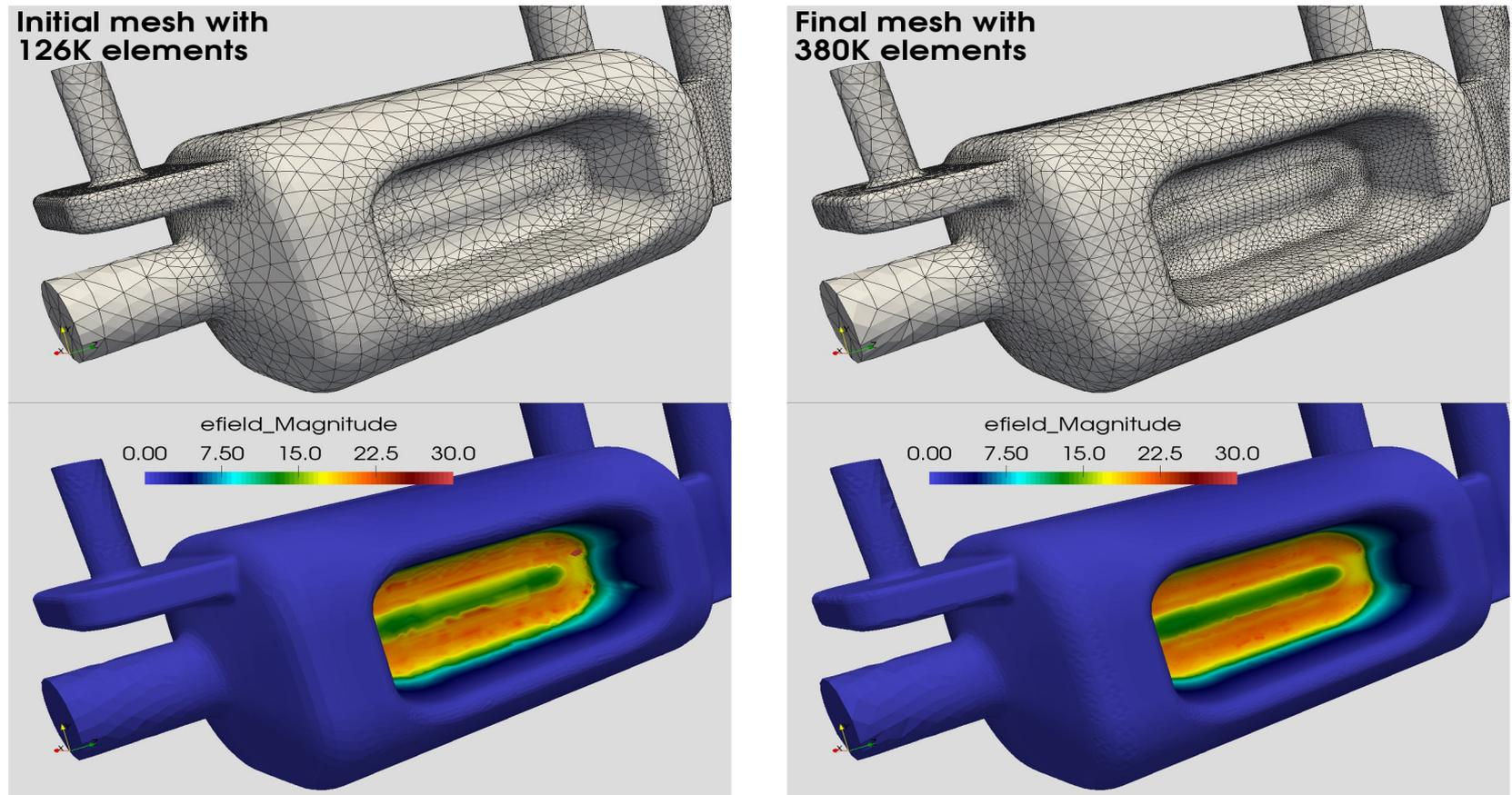
*This figure shows the adaptation results for the CAV17 model. (top left) shows the initial mesh with ~126K elements, (top right) shows the final (after 3 adaptation levels) mesh with ~380K elements, (bottom left) shows the first eigenmode for the electric field on the initial mesh, and (bottom right) shows the first eigenmode of the electric field on the final (adapted) mesh.*
