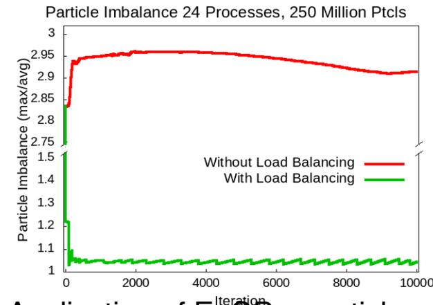
Application of EnGPar particle dynamic load balancing in a GITRm impurity transport simulation
