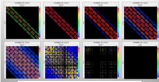
Performance degradation caused by increased communication complexity on coarser grids!
