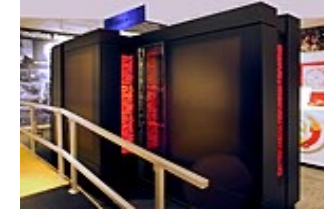
Thinking Machines' CM-5. 1K SPARC CPUs SIMD. Fat Tree.
