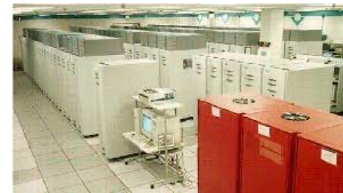
ASCI Red, Intel-Sandia 'partitioned' design. x86 CPUs. First Teraflops system on Top500 ('96)
