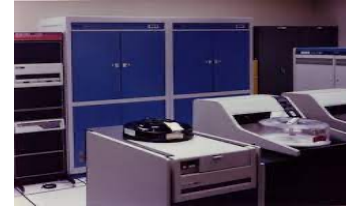
Goodyear MPP. 16K 1-bit CPUs SIMD
