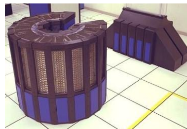
Cray-2. Decisively broke the GF barrier.
