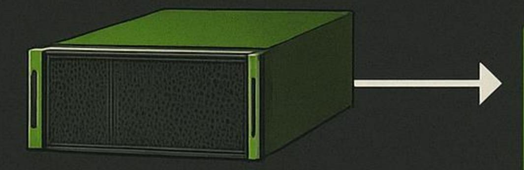
DGX SYSTEM Purpose-built Al server Contains 8 GPUs or multiple superchips Includes networking, storage, and cooling in one chassis
